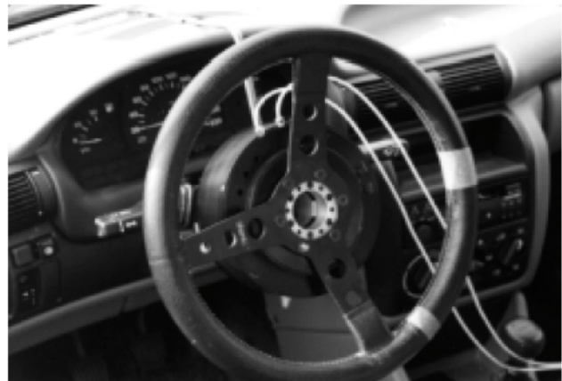
Mounting principle of transducer on steering column - no disassembly of column is required. Adapters are not supplied
